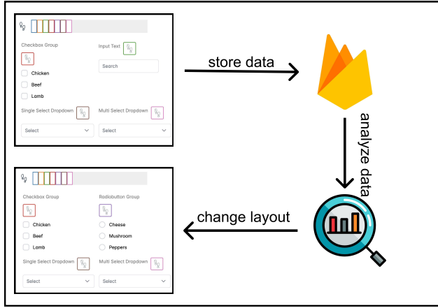
Figure 7: High-level process diagram for offline UI layout customization.
